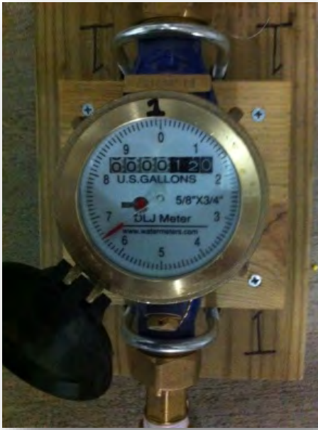
Figure 2. Two water meters purchased and installed on March 20 th , 2014 to measure pen wash down water additions to manure volume. Initial meters readings were 126.6 and 80.2 gallons for meter 1 and 2.
