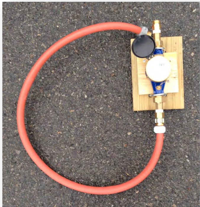
Figure 1. Standard water meter with hose adapters and mounting base installed to measure water use during pressure washing to clean animal pens.
