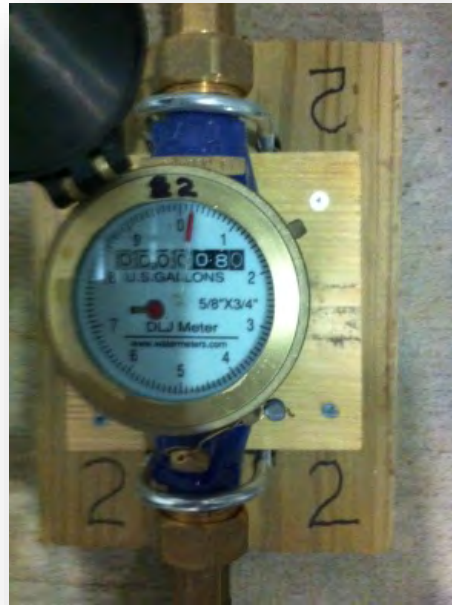
Figure 2. Two water meters purchased and installed on March 20 th , 2014 to measure pen wash down water additions to manure volume. Initial meters readings were 126.6 and 80.2 gallons for meter 1 and 2.
